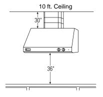
**9 ft. ceilings:** When the hood is installed 30" above the cooking surface, order two 12" duct cover accessories.
